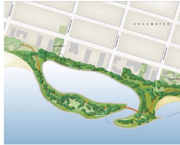
An alternate Edgewater proposal creates two peninsulas enclosing a new lagoon, with a bridge for the lakefront path.
